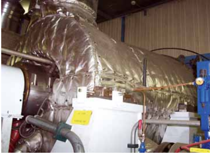
Matelas haute température - Application TAV et TAG High Temperature stuffing mats - Application: Gas & Steam Turbine
