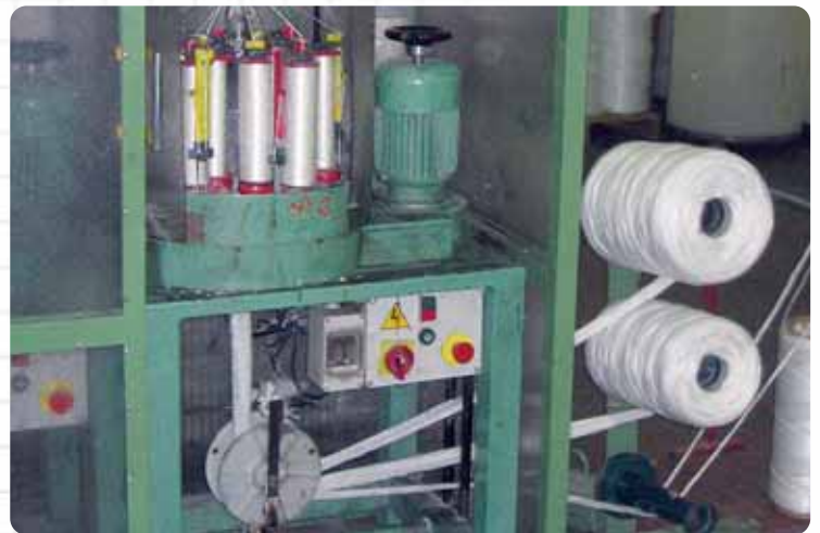
Corde/tresse de verre HT - 800°C Rope/HT braided glass - 800°C
